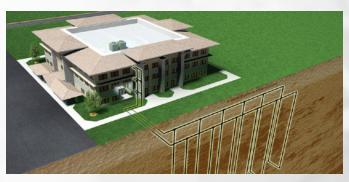
HYBRID LOOP: Combines boiler tower and geothermal loop technologies to achieve optimal efficiencies, while meeting the challenges of both loop field space and budget constraints.
